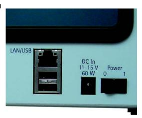
The 2303 Stabilock can be operated either from the internal battery or from an external DC source such as the power supply which is delivered with the 2303, or a car battery. The DC voltage must be in the range from 11 to 15 V. In addition, the battery is loaded when an external DC source is connected.
