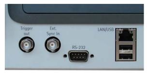
This 9-pin sub-D connector on the rear panel of the 2303 Stabilock can be used to control the 9100 remotely via serial interface (RS-232). The command set and the responses conform to the SCPI standard and are explained in the user's guide.
