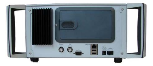
The 2303 Stabilock can be equipped with a rechargeable battery module to enable operation in the field, without mains voltage. If you ordered your 2303 with a battery, that battery will already be installed. This battery must be charged before first-time use. Please allow six hours to charge while the instrument is connected to an external power supply and switched off.
